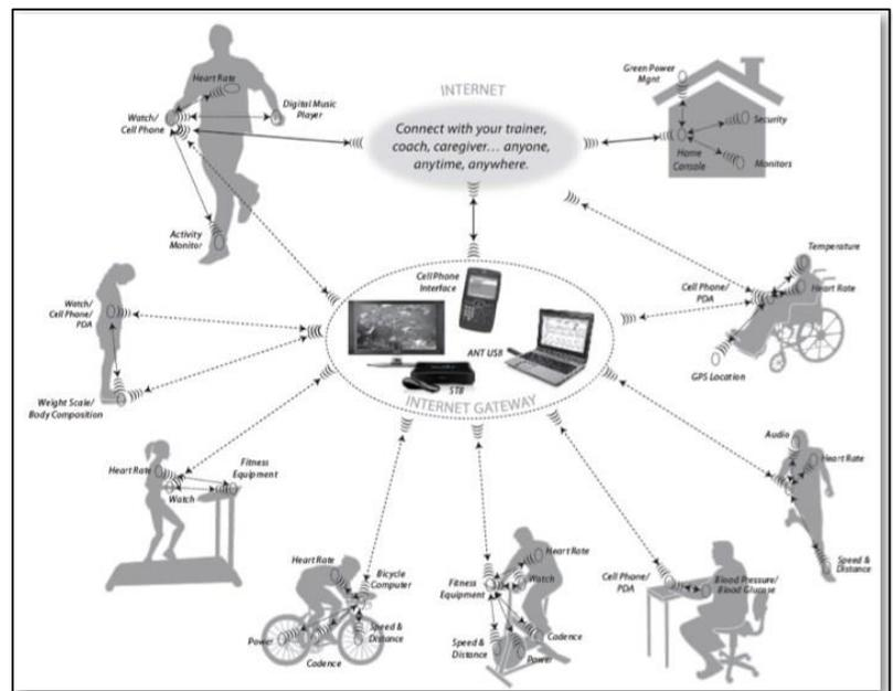
Figure 1: Multiple Device Collection System Using ANT+
